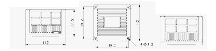
Note: Unfilled dimensional tolerances are performed in accordance with GB/T1804-2000 Class C.
