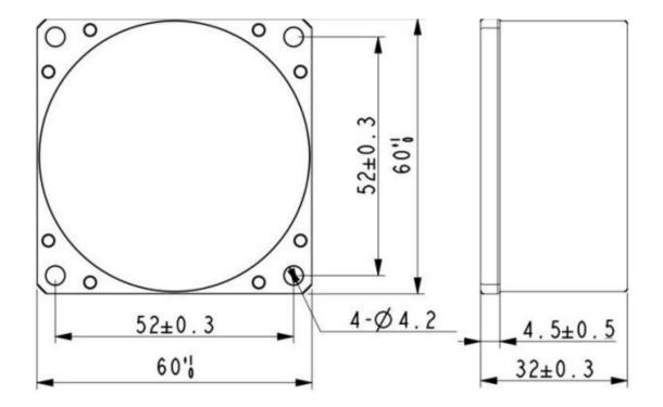
Note: Unfilled dimensional tolerances are performed in accordance with GB/T1804-2000 Class C.
