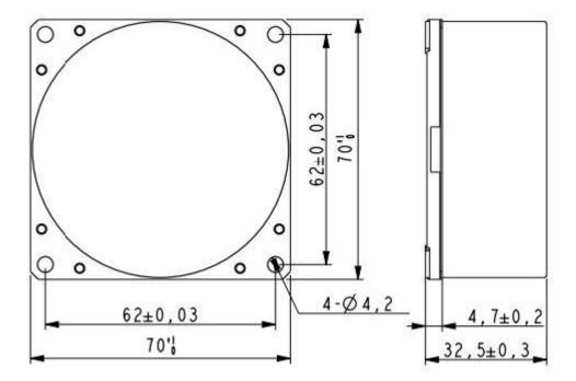
Note: Unfilled dimensional tolerances are performed in accordance with GB/T1804-2000 Class C.
