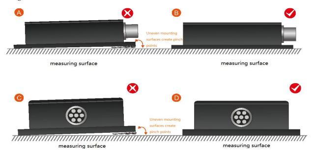
Secondly, the bottom line of the sensor and the axis of the measured object cannot have an angle as shown in Figure E, and the bottom line of the sensor should be kept parallel or orthogonal to the axis of rotation of the measured object during installation. This product can be installed horizontally or vertically (vertical installation needs to be customized), and the correct installation method is shown in Figure F.
