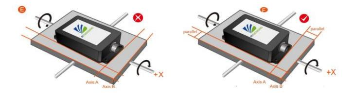
Finally, the mounting surface of the sensor and the surface to be measured must be tightly fixed, smooth in contact, and stable in rotation, and measurement errors due to acceleration and vibration must be avoided.
