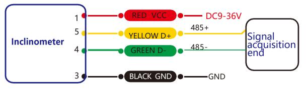
RS 485 wiring diagram
