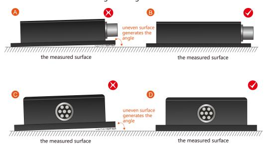
Finally, after the product is tightly attached, screws should be used to fix the IMU to ensure tight fixation, smooth conduct and stable rotation. Measurement errors caused by acceleration and vibration should be voided. Bear in mind that the screw only plays a fixed role and doe not have a positioning function. The screw hole of the IMU is processed into an elliptical shape for easy adjustment.
