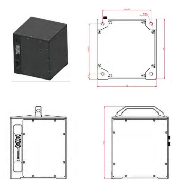
Note: Unfilled dimensional tolerances are performed in accordance with GB/T1804-2000 Class C.
