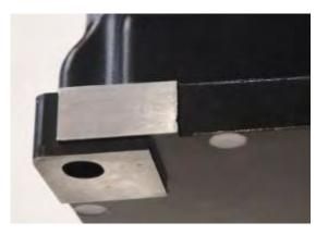
First of all, to ensure that the sensor mounting surface and the measured surface completely close, the measured surface should be as horizontal as possible, so that we can reduce installation error.
