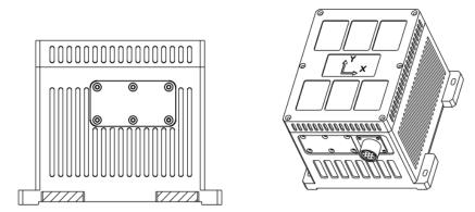
Note: Unfilled dimensional tolerances are performed in accordance with GB/T1804-2000 Class C.
