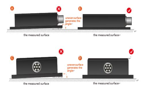
Secondly, the bottom line of the sensor and the axis of the measured object cannot have an angle as shown in Figure E. When installing, keep the bottom line of the sensor parallel or orthogonal to the axis of rotation of the measured object. This product can be installed horizontally or vertically (vertical installation needs to be customized), and the correct installation method is shown in Figure F.
