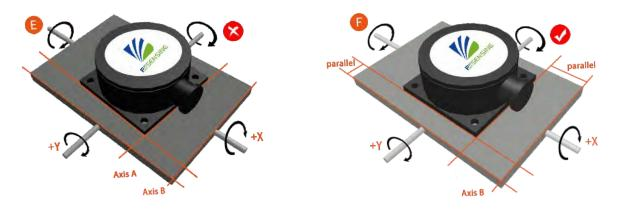
Finally, the mounting surface of the sensor and the surface to be measured must be tightly fixed, smooth in contact, and stable in rotation, and measurement errors due to acceleration and vibration must be avoided.
