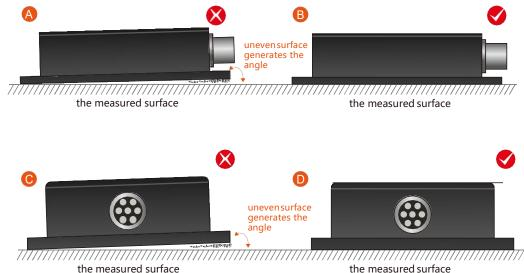
Secondly, the bottom line of the sensor and the axis of the measured object cannot have an angle as shown in Figure E, and the bottom line of the sensor should be kept parallel or orthogonal to the axis of rotation of the measured object during installation. This product can be installed horizontally or vertically (vertical installation needs to be customized), and the correct installation method is shown in Figure F.
