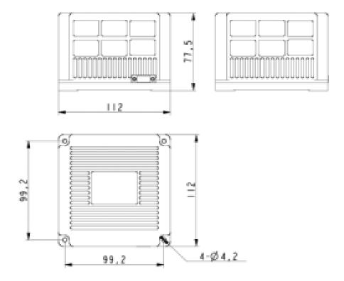
Note: Unfilled dimensional tolerances are performed in accordance with GB/T1804-2000 Class C.
