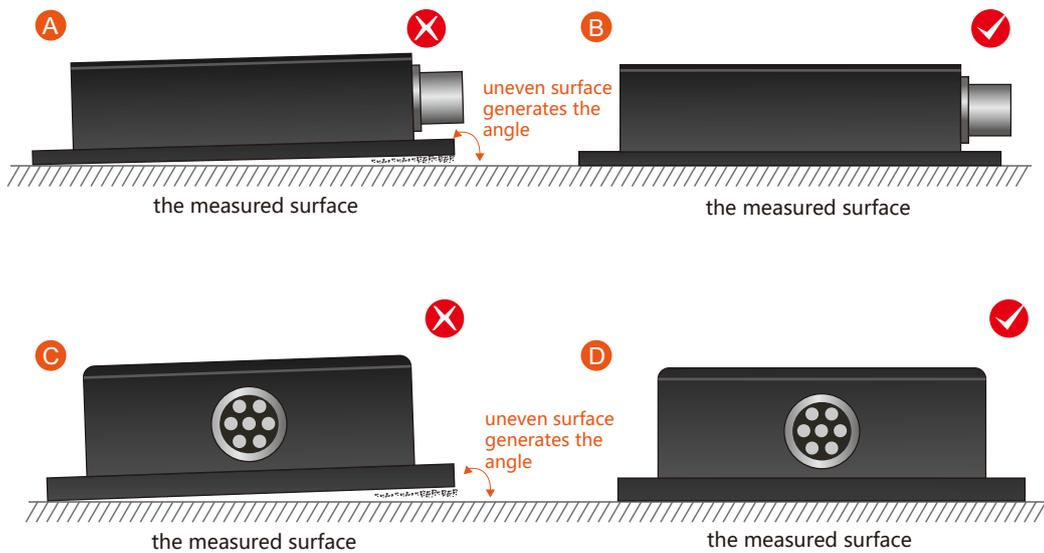
Secondly, the bottom cable of the sensor and the axis of the measured object shouldn't generate the angle shown in E. When installing, the bottom cable of the sensor should be kept parallel or orthogonal to the rotation axis of the measured object. This product can be installed horizontally or vertically (vertical installation requires customization). The correct installation method is shown in Figure F.
