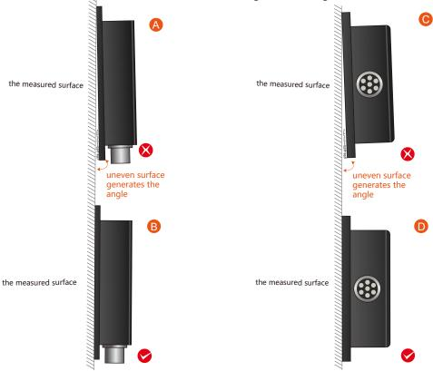
Secondly, the bottom cable of the sensor and the axis of the measured object shouldn't generate the angle shown in E. When installing, the bottom cable of the sensor should be kept parallel or orthogonal to the rotation axis of the measured object. This product can be installed horizontally or vertically (vertical installation requires customization). The correct installation method is shown in Figure F.
