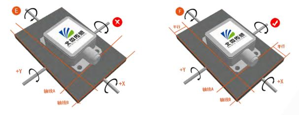
Finally, the installation surface of the sensor must be fixed with the measured surface tightly and smoothly, to avoid measurement error that may be caused by the acceleration and vibration.
