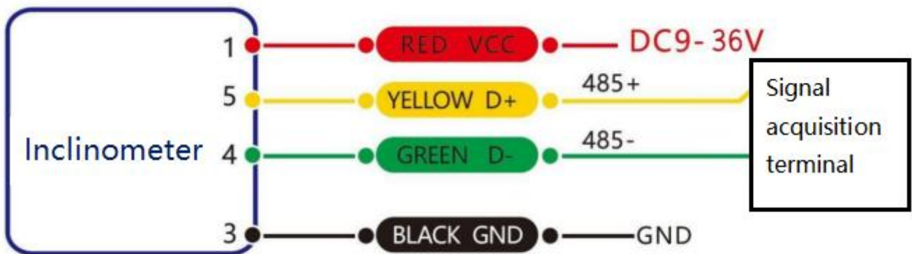
RS 485 wiring diagram
