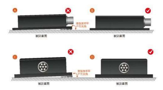
Secondly, the bottom line of the sensor and the axis of the measured object cannot have an angle as shown in Figure E, and the bottom line of the sensor should be kept parallel or orthogonal to the axis of rotation of the measured object during installation. This product can be installed horizontally or vertically (vertical installation needs to be customized), and the correct installation method is shown in Figure F.
