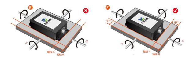
Finally, the mounting surface of the sensor and the surface to be measured must be tightly fixed, smooth in contact, and stable in rotation, and measurement errors due to acceleration and vibration must be avoided.
