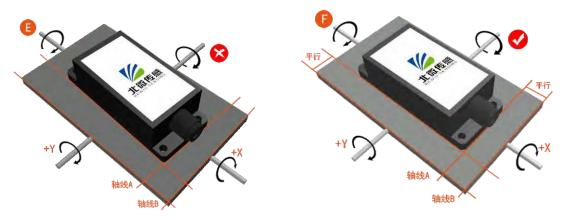
Finally, the mounting surface of the sensor and the surface to be measured must be tightly fixed, smooth in contact, and stable in rotation, and measurement errors due to acceleration and vibration must be avoided.
