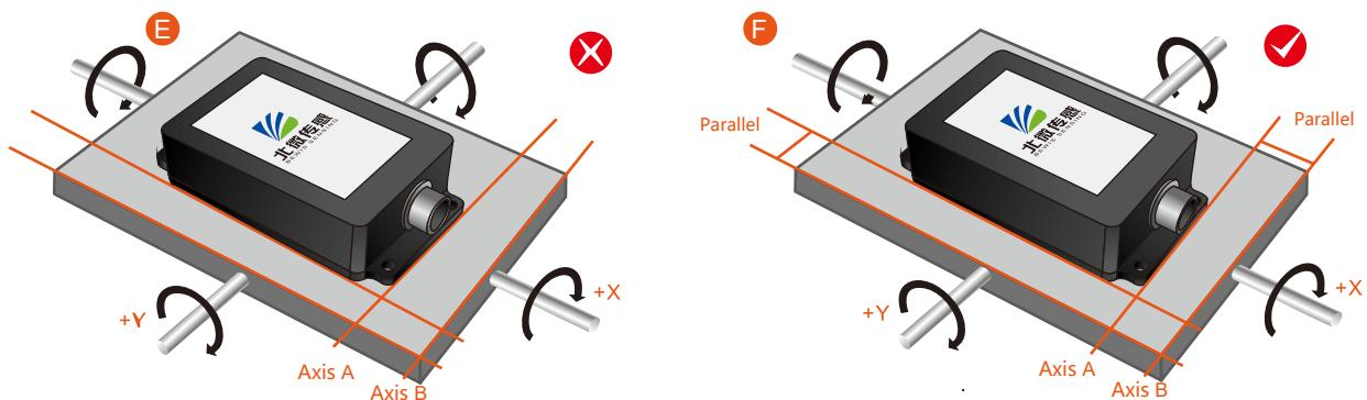
Finally, the installation surface of the sensor must be fixed with the measured surface tightly and smoothly, to avoid measurement error that may be caused by the acceleration and vibration.
