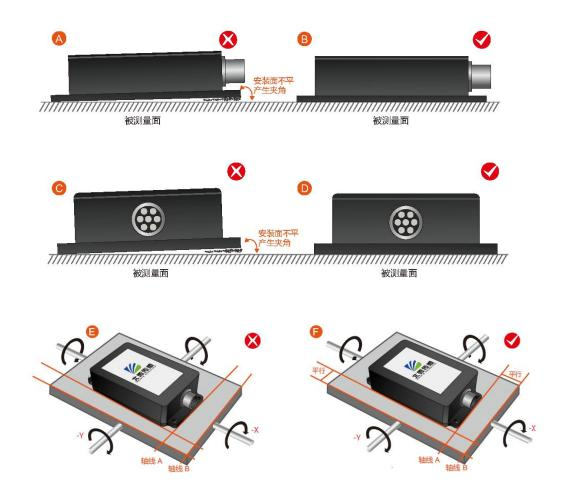
Keep away from strong magnetic field materials such as magnets, iron, and nickel to prevent irreversible damage to the product's magnetic-sensitive components. Keep clear of motors, wires, capacitors, inductors, and other components that generate magnetic fields due to current flow. This prevents continuous measurement from being affected by electromagnetic field fluctuations caused by energised components, thereby safeguarding the sensor's heading accuracy.
