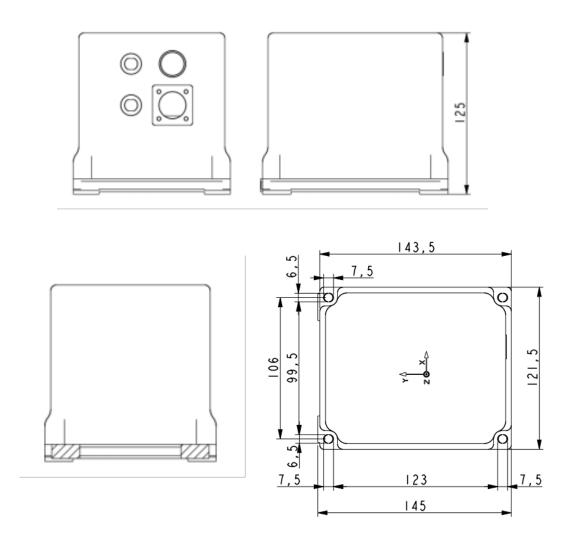
Note: Unfilled dimensional tolerances are performed in accordance with GB/T1804-2000 Class C.
