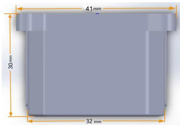
Note: Unfilled dimensional tolerances are performed in accordance with GB/T1804-2000 Class C.
