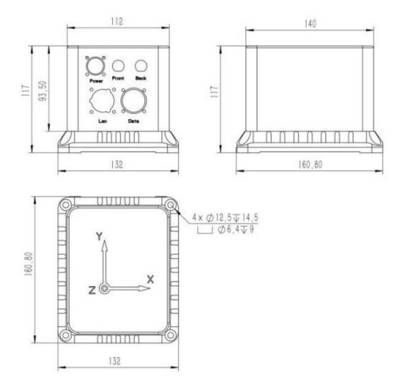
Note: NO dimension tolerance is specified according to grade C of GB/T1804-2000.
