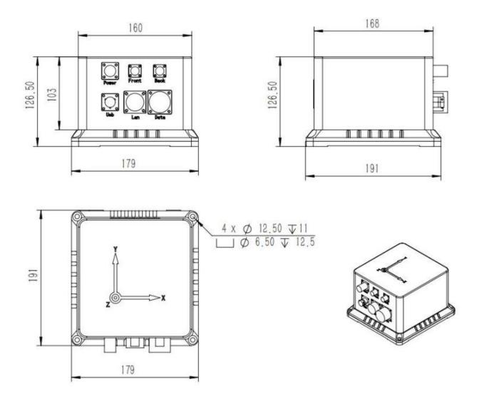
Note: NO dimension tolerance is specified according to grade C of GB/T1804-2000.
