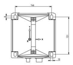
Note: NO dimension tolerance is specified according to grade C of GB/T1804-2000.
