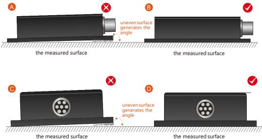
Finally, after the integrated navigation system is closely attached to the body, use screws to ensure tight fixation, smooth contact, stable rotation, and avoid measurement errors due to acceleration and vibration. Remember that at this time, the screw only serves as a fixing function, not a positioning function. The screw hole of the integrated navigation system is processed into an oval shape for easy adjustment.
