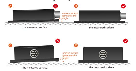
Finally, after the product is tightly attached, screws should be used to fix the IMU to ensure tight fixation, smooth conduct and stable rotation. Measurement errors caused by acceleration and vibration should be voided. Bear in mind that the screw only plays a fixed role and doe not have a positioning function. The screw hole of the IMU is processed into an elliptical shape for easy adjustment.
