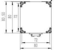
Attention: Unmarked dimensional tolerance is implemented according to GB/T1804-2000 grade C
