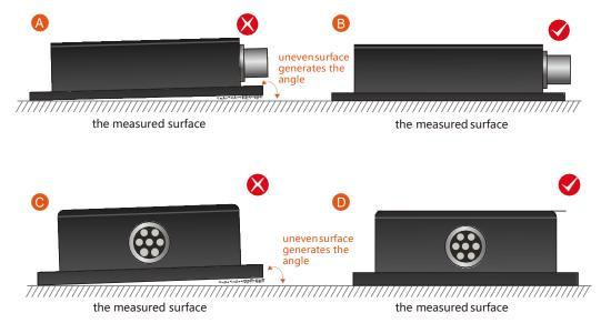
Finally, after the integrated navigation system is closely attached to the body, use screws to ensure tight fixation, smooth contact, stable rotation, and avoid measurement errors due to acceleration and vibration. Remember that at this time, the screw only serves as a fixing function, not a positioning function. The screw hole of the integrated navigation system is processed into an oval shape for easy adjustment.
