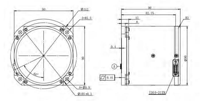
Note: Unfilled dimensional tolerances are performed in accordance with GB/T1804-2000 Class C.
