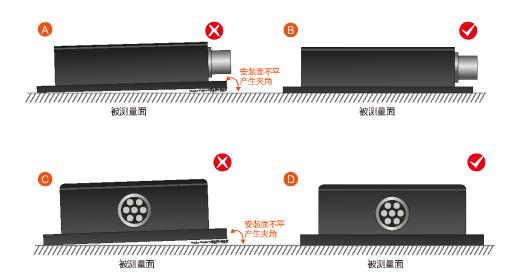
Secondly, the bottom line of the sensor and the axis of the measured object cannot have an angle as shown in Figure E. When installing, keep the bottom line of the sensor parallel or orthogonal to the axis of rotation of the measured object. This product can be installed horizontally or vertically (vertical installation needs to be customized), and the correct installation method is shown in Figure F.
