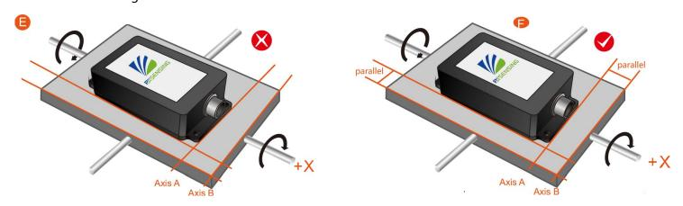
Finally, the mounting surface of the sensor and the surface to be measured must be tightly fixed, smooth in contact, and stable in rotation, and measurement errors due to acceleration and vibration must be avoided.
