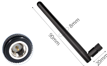
9cm 2.5dBi antenna *1PC(Optional) Two types of antennas can be chosen to meet the needs of frequency band switching (848-888MHz) or (895-935MHz)
