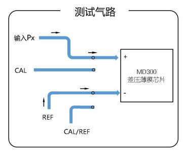
The gas route in the test environment has 8 input terminals Px and the differential pressure common pressure terminal REF. The gas path is switched to the test environment through the front PA piston air nozzle, the test pressure is directly input to the differential pressure chip through the upper air nozzle, and then the differential pressure is input to the pressure chamber through the atmospheric pressure to complete the differential pressure comparison and obtain the complete data.
