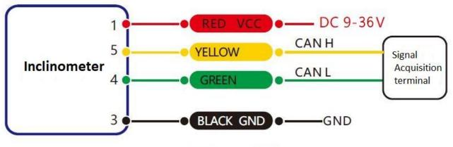
CAN bus wiring diagram
