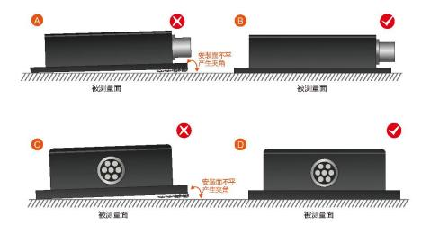
Secondly, the bottom edge line of the sensor and the axis of the measured object cannot have the angle shown in Figure E, and the installation should keep the bottom edge line of the sensor parallel or perpendicular to the rotating axis of the measured object. This product can be installed horizontally or vertically (vertical installation requires customization), and the correct installation method is shown in Figure F.
