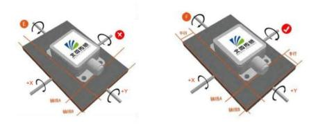
Finally, the mounting surface of the sensor and the measured surface must be fixed tightly, smooth contact, and stable rotation, to avoid measurement errors caused by acceleration and vibration.
