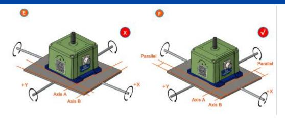
Finally, the mounting surface of the sensor and the surface to be measured must be tightly fixed, smooth in contact, and stable in rotation, and measurement errors due to acceleration and vibration must be avoided.
