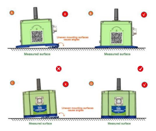
Secondly, the bottom line of the sensor and the axis of the measured object cannot have an angle as shown in Figure E, and the bottom line of the sensor should be kept parallel or orthogonal to the axis of rotation of the measured object during installation. This product can be installed horizontally or vertically (vertical installation needs to be customized), and the correct installation method is shown in Figure F.
