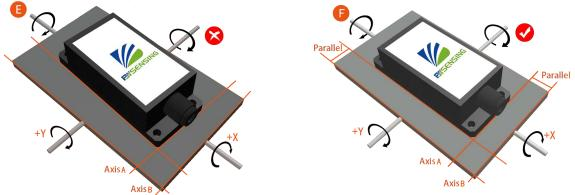
Finally, the installation surface of the sensor must be fixed with the measured surface tightly and smoothly, to avoid measurement error that may be caused by the acceleration and vibration.
